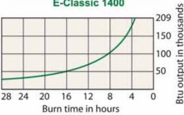
Based on EPA output ratings. Actual Btu output and burn time will be affected by the type of wood burned, its moisture content and other factors.
